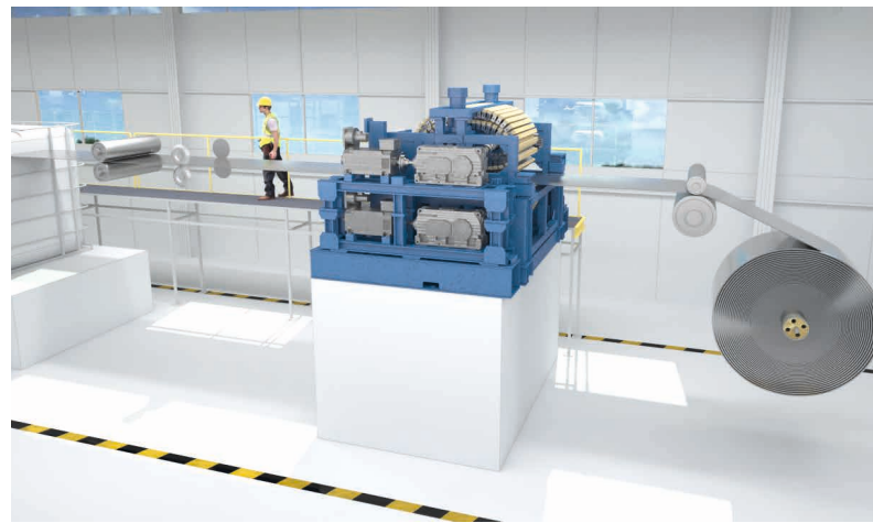
The third Umlauf Bridle, arranged at the run-out, creates the back-tension needed to produce exactly wound coils
