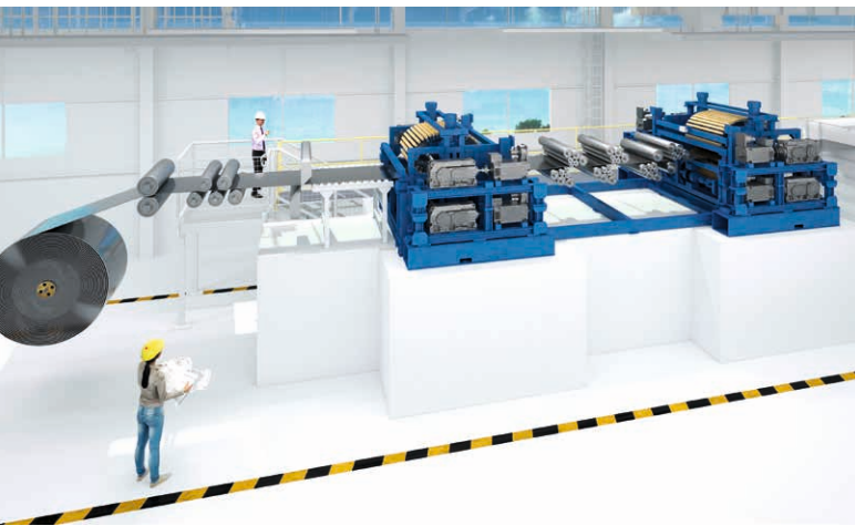
The first unit is arranged directly behind the pay-off reel; the second one pushes the leveled strip into the pickling tank
